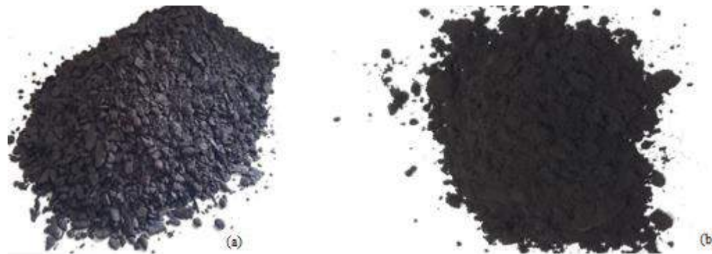
Figure 1. A Photographic View of Coal Particles Before (a) and After (b) Milling Process
