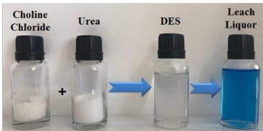
Figure 1. The Prepared Deep Eutectic Solvent and Leach Liquor Obtained After Leach Process at 95 °C Reaction Temperature, 1/20 Solid-to Liquid Ratio and 48 Hours.
