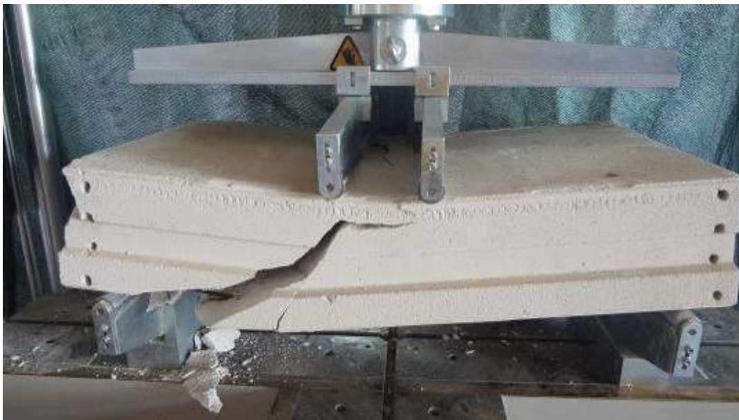
Figure 5 Failed RAACP (monotonic loading)
