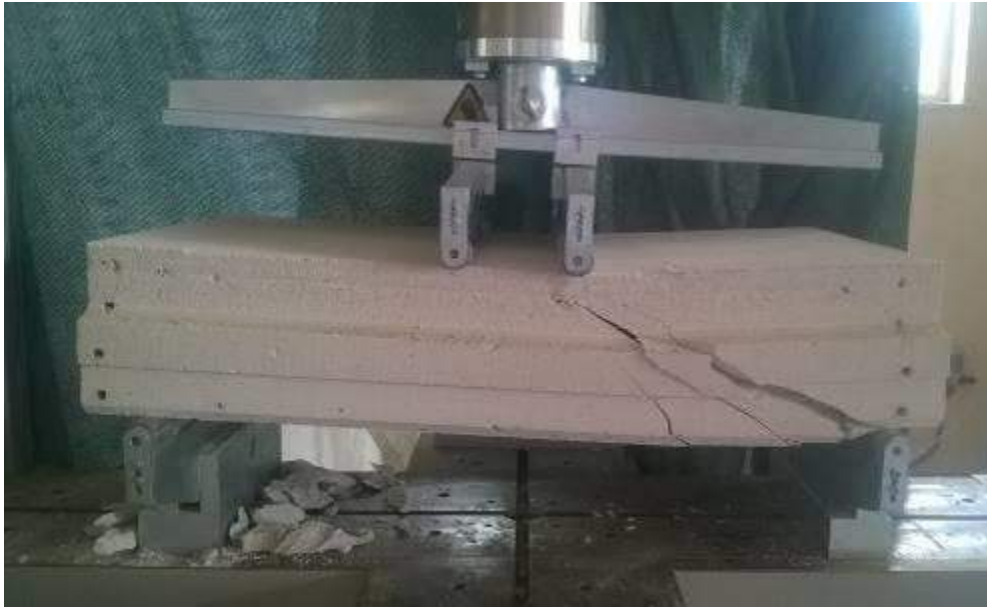
Figure 4 Failed RAACP (cyclic loading)
