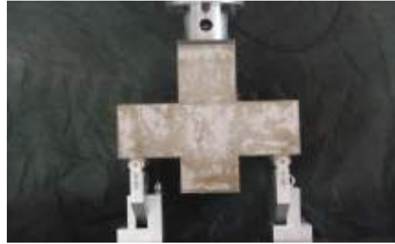
Figure 2 Test Configuration and Set-up for Corbels
