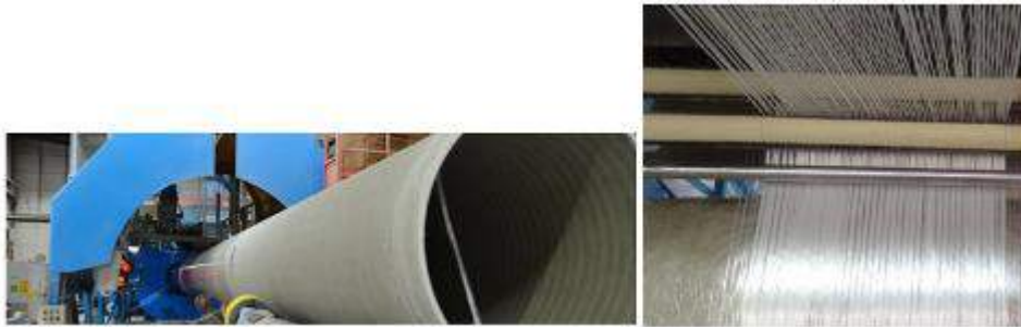
Figure 1. Continuous filament winding technique
