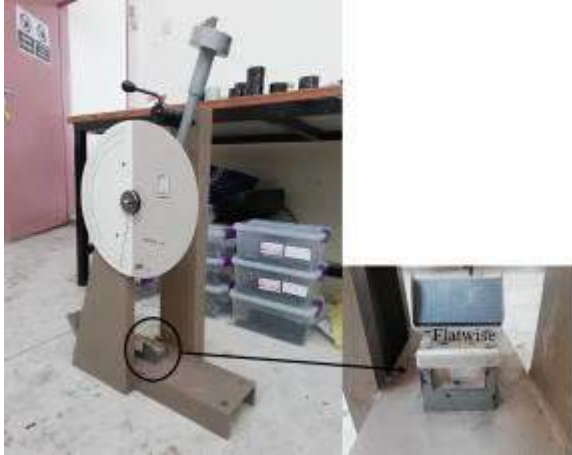
Figure 3. Kögel 3/70 Charpy impact tester
